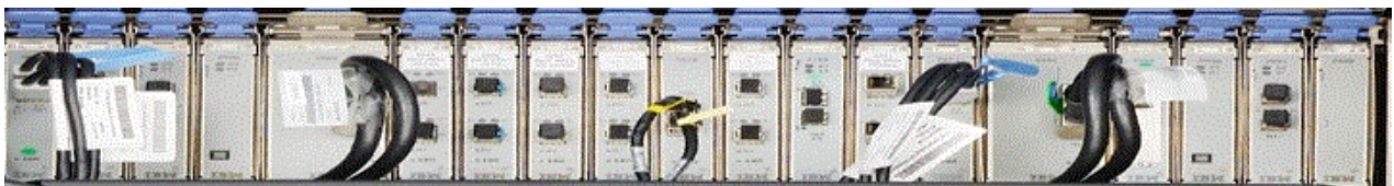
Figure 43. Photograph of a physical adapter card in a system I/O drawer
